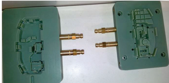
Core and cavity mold inserts ready for assembly onto the molding machine together with fittings for cooling lines.
